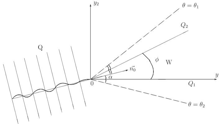
Figure 1. Scattering on a wedge.
