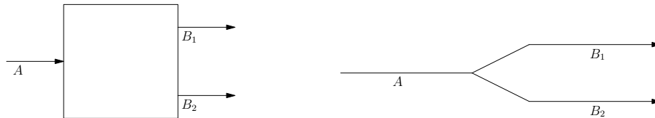
Figure 4: Graphical and simplified graphical representation of the divider (left and right, respectively) with inlet A and outlets B_1 and B_2 .
