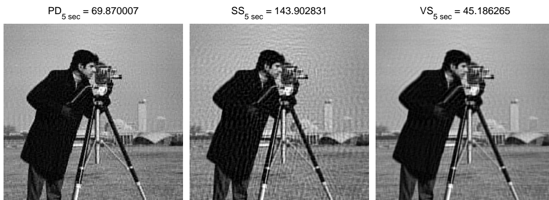
Figure 4.2: Results furnished by the primal-dual (PD), the skew splitting (SS) and the variable smoothing (VS) algorithms after 5 seconds of CPU time.
