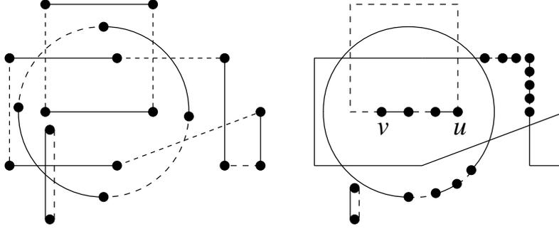
**FIG. 8.** (d) Move the vertices along each curve till they're all between 2 crossings; now they're also in one planar region w.r.t. all other cycles.
